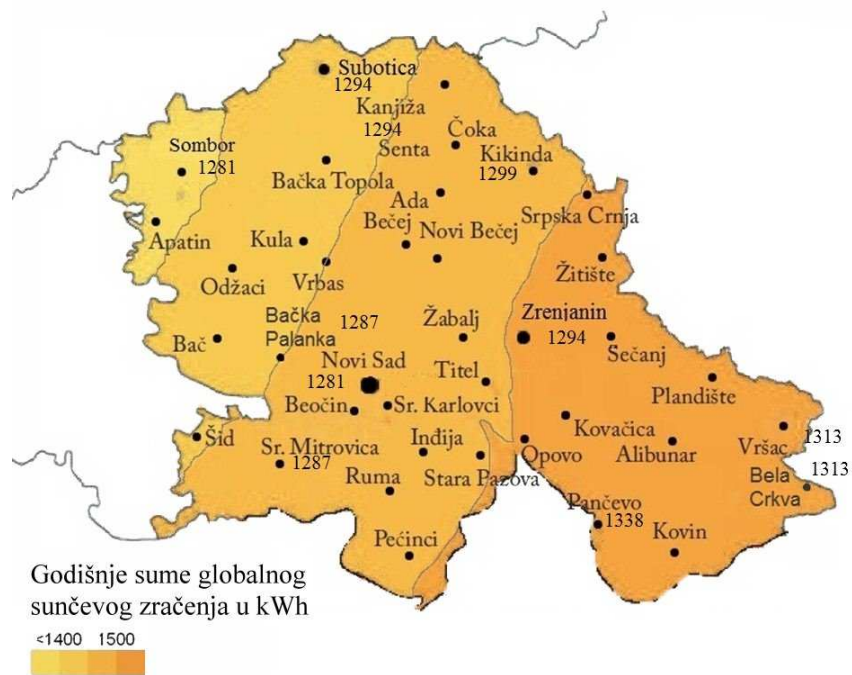
Yearly average of daily global energy radiation (in kWh/m 2 ) on horizontal surface (0°) for Vojvodina
