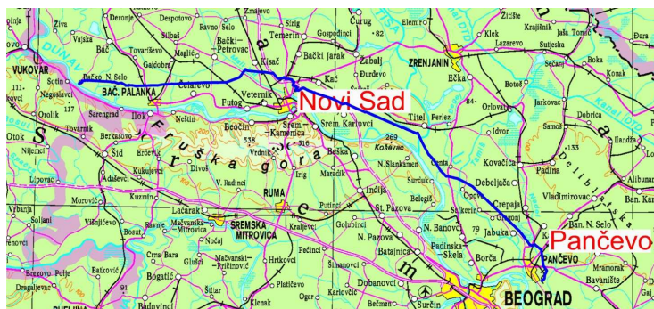
Figure 5.3: Route of the Pipeline the Danube - Bačko Novo Selo - Novi Sad – Pančevo along which an optical cable will be laid down
